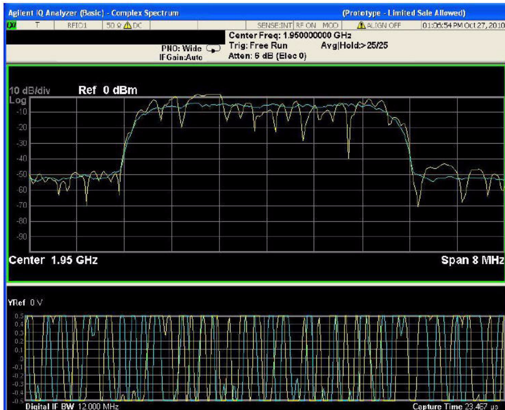
Figure 11-16. Verifying the “All Up” Uplink Signal
